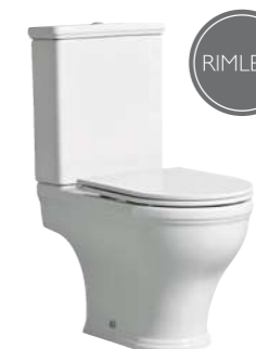
Lansdown Short Projection Open Back Close Coupled WC Spigot distance from wall 137mm 360(w) x 845(h) x 620(d)mm Pan - DC14043 6/4L Cistern - DC14036 Seat - DC14037
