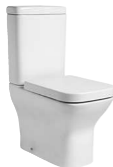
Fully Enclosed Close Coupled WC Spigot distance from wall 150mm 345(w) x 850(h) x 610(d)mm Pan - PF450S 4.5/3L Cistern - C450S Seat - TS450S
