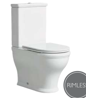
Short Projection Fully Enclosed Close Coupled WC Spigot distance from wall 137mm 360(w) x 845(h) x 620(d)mm Pan - DCI14042 6/4L Cistern - DCI14036 Seat - DCI14037 Total
