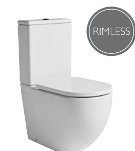
Orbit Fully Enclosed Close Coupled WC Spigot distance from wall 190mm 370(w) x 835(h) x 620(d)mm Pan - P250S 4.5/3L Cistern - RA453CCC Seat - TS250S-SF
