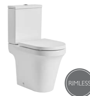
Comfort Height Open Back Close Coupled WC With Contactless Flush Spigot distance from wall 160mm 395(w) x 875(h) x 620(d)mm Pan - PC650S Sensor Cistern - C650S-SEN Seat - TS650S
